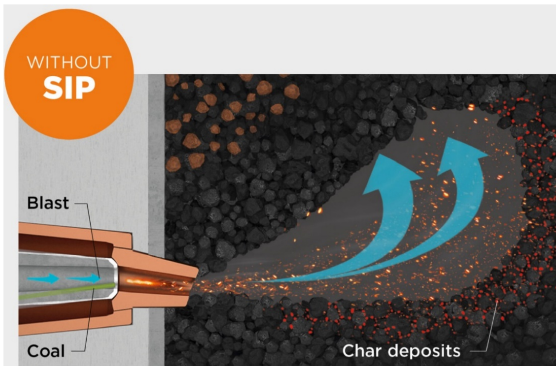
Fig. 1. Carbon injection in BF without SIP
