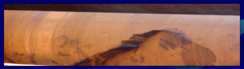
• BANDING/PEELING (harmful for strip rolling, lead to rolled in scale along with roll).
