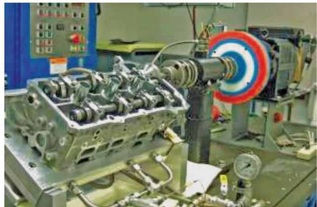
Fig. 3—The motored valve train rig for friction evaluation.
