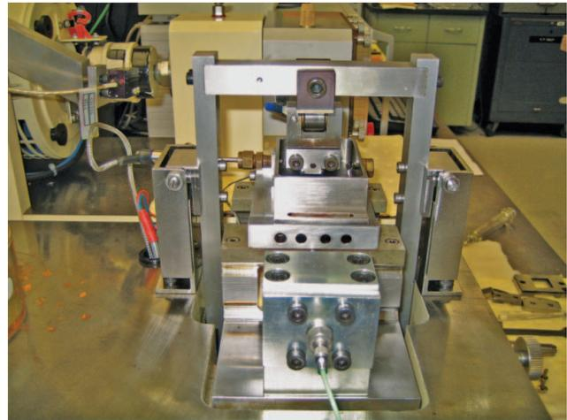
Fig. 2—The Plint test machine used for friction and wear evaluation under boundary lubrication conditions.
