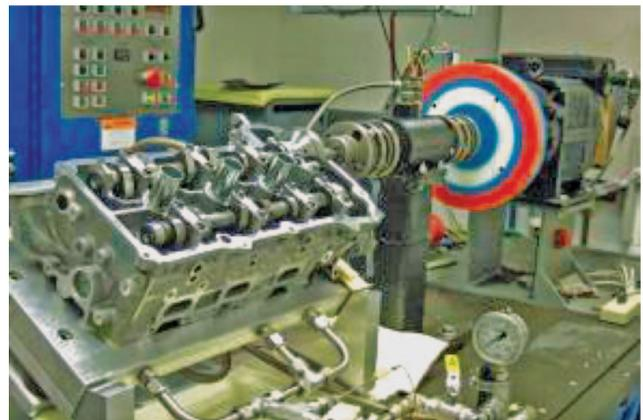
Fig. 3—The motored valve train rig for friction evaluation.
