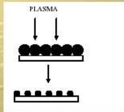
2. Remove nanospheres leaving hexagonal array of holes in a metal film
