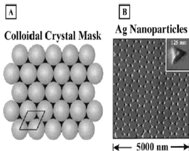
**Figure 1.** Schematic illustration (A) and representative AFM image (B) of SL PPA. The ambient contact mode AFM image was captured from a SL PPA fabricated with  $D = 542$  nm nanospheres and  $d_m = 48$  nm thermally evaporated Ag metal after 3 min sonication in methylene chloride.
