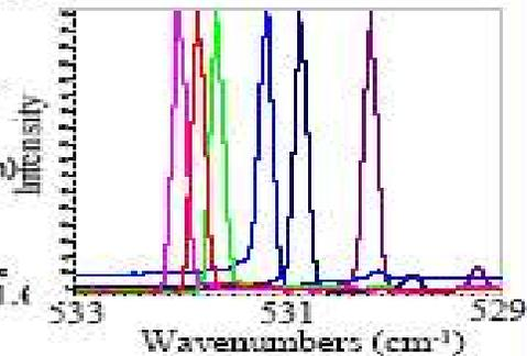
Spectral tuning of nearly circular ( $\epsilon = 0.027$ ) laser for increasing current.
