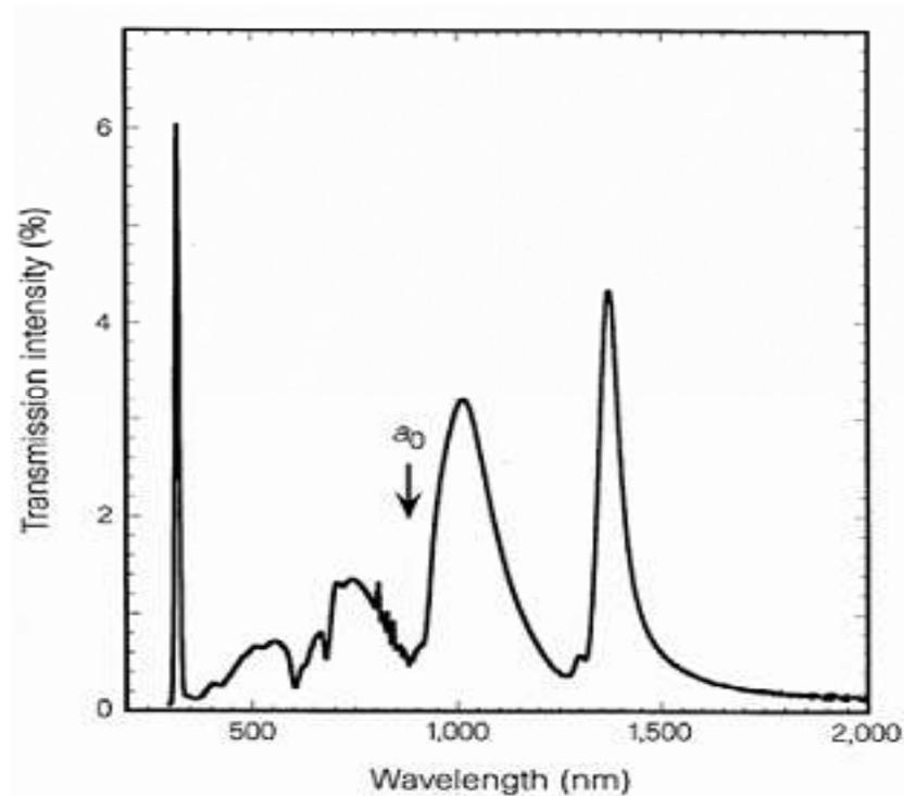
3. Zero-order transmission spectrum for a square array of 150 nm holes with a period of 900 nm in a 200 nm thick Ag film. The maximum transmitted intensity occurs at 1370 nm, nearly ten times the diameter of an individual hole in the array (Ebbesen 1998).
