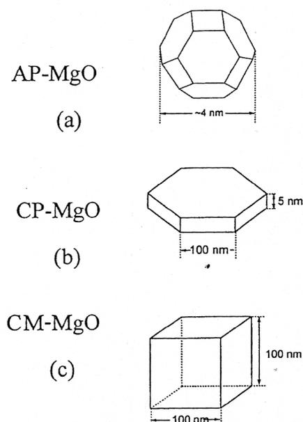
Models of (a) nanocrystalline (AP-MgO); (b) microcrystalline (CP-MgO); (c) normal commercially available (CM-MgO) magnesium oxide crystals. Reprinted with permission from *Clusters & Nanostructure Interfaces*, 1999, p. 578, World Scientific Publishing Co Pte Ltd.<sup>1b</sup>
