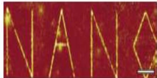
THIN LAYER OF SILVER acts like a superlens over very short distances. Here the word "NANO" is imaged with a focused ion beam (*left*), optically without a superlens (*middle*) and optically with
