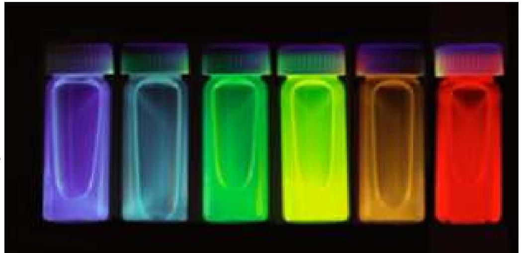
Colloidal CdSe quantum dots dispersed in hexane
