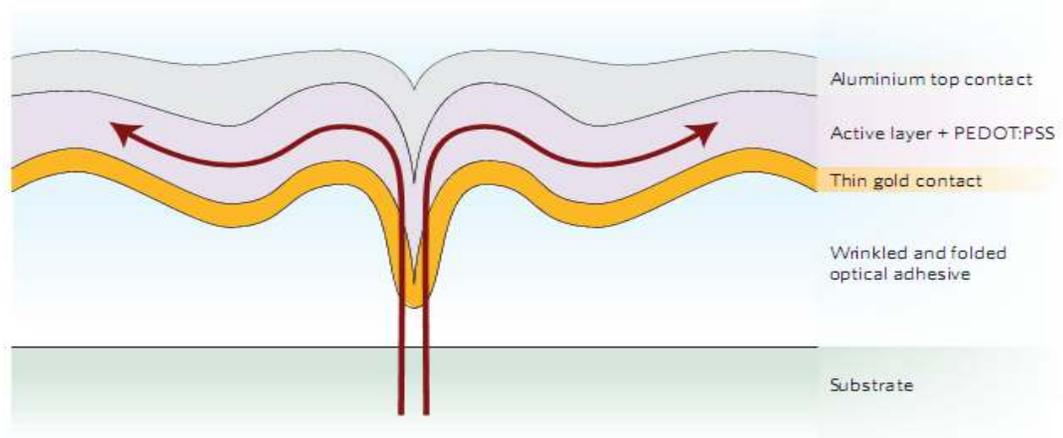
**Figure 1** | Long-wavelength photons propagating across a wrinkled and folded substrate. Photons incident on the substrate side get 'folded' into the active layer of the cell by the folds in the polymer adhesive. The wrinkles further localize the light inside the layer through waveguiding effects. PEDOT:PSS, poly(3,4-ethylenedioxythiophene) poly(styrenesulphonate).
