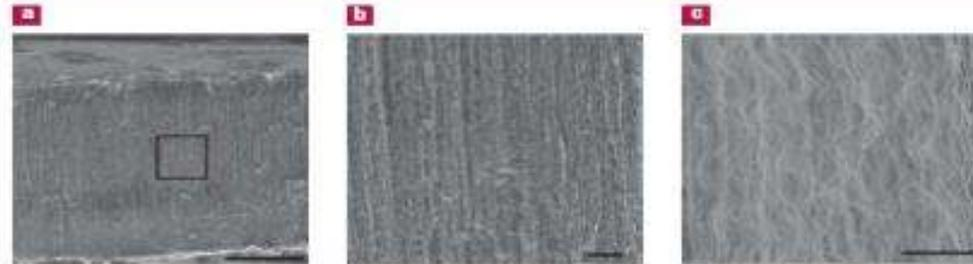
Structural characterization of macro tubes made from MWNT
