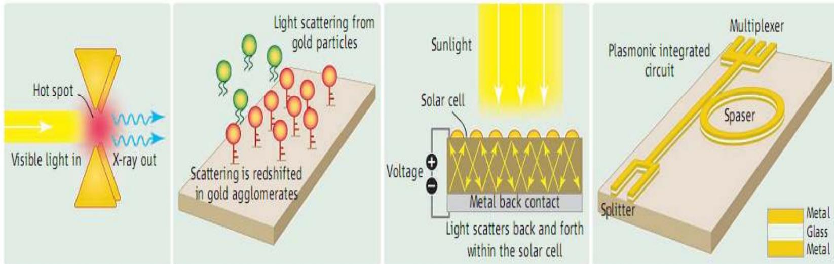
**Applied plasmonics.** (Left) A plasmonic hot spot between metal nanoparticles creates soft x-rays. (Middle left) Measuring the resonance shift in coupled metal nanoparticles leads to efficient sensing. (Middle right) Scattering from
