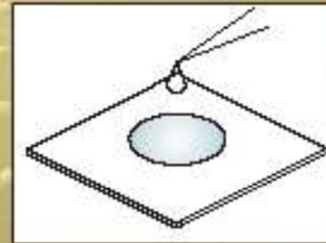
2. Dry in oven, spheres self-assemble at meniscus edge
