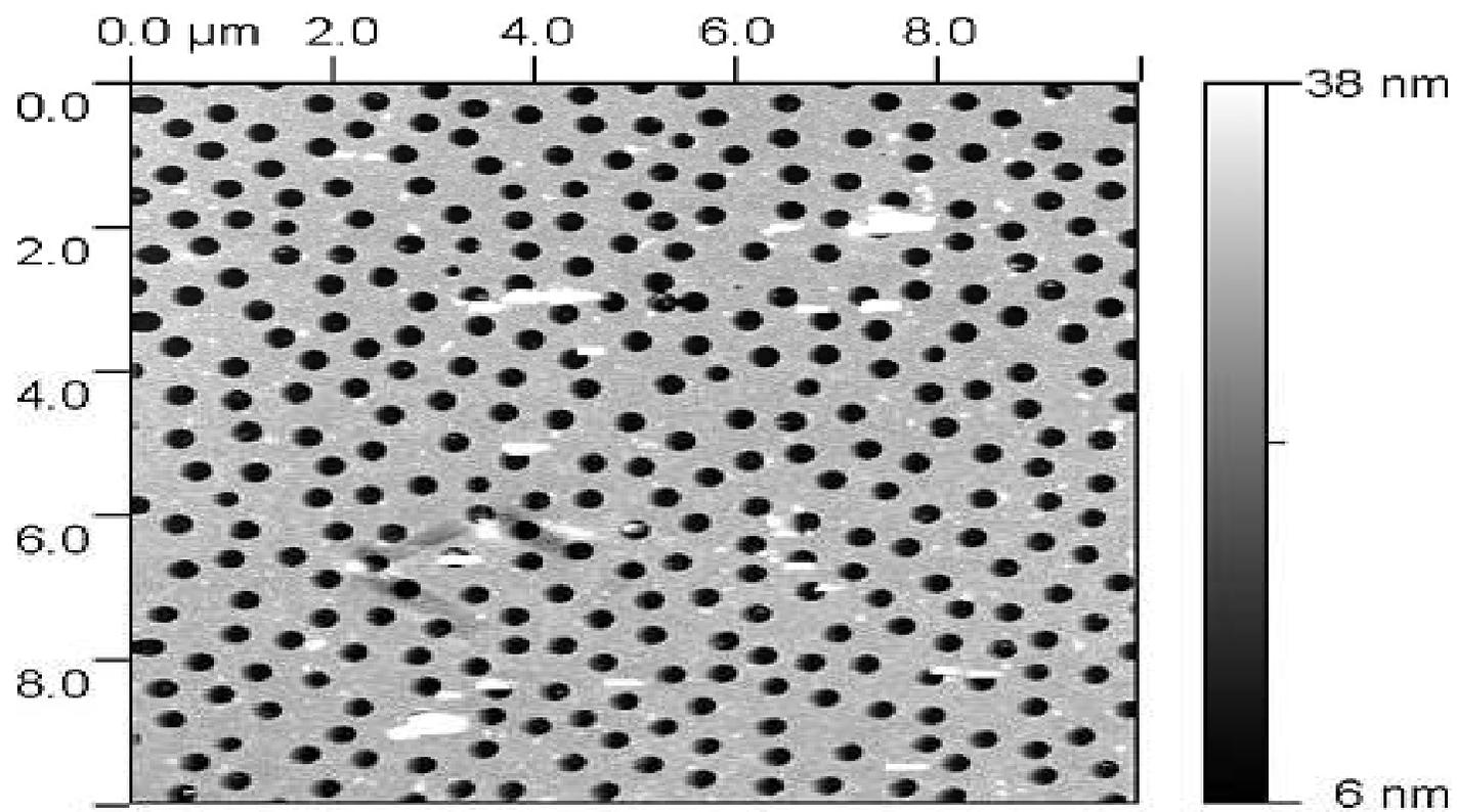
FIG. 1. Atomic force micrograph of 30-nm silver nanohole film fabricated by the colloidal lithography method using 350-nm latex spheres.
