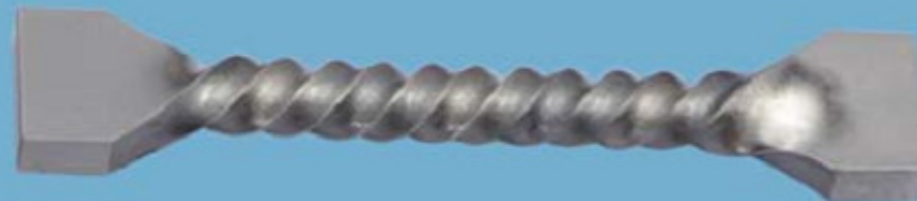
Sample after twisting by 1080° (T = 20 °C)
