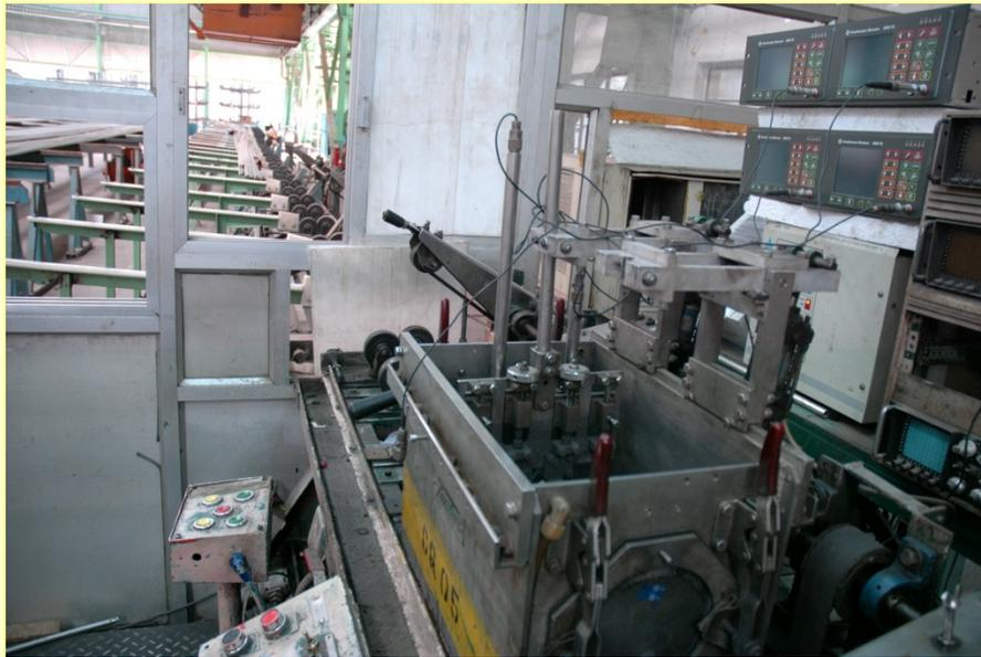
Automated Ultrasonic Testing Unit
