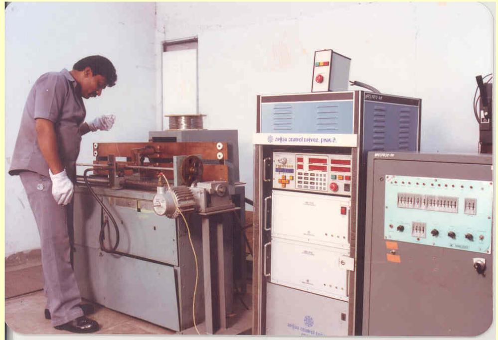
**Wire-Wrap Machine for Radial Blanket Pin**
