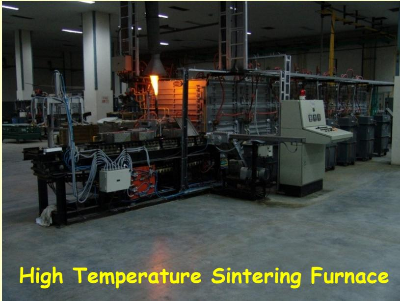
**High Temperature Sintering Furnace**
